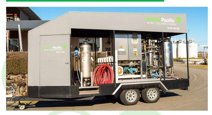
Memstar (Membrane Separation Treatment And Removal) is a family of membrane-based processes for adjusting wine composition and enhancing quality. These technologies are offered in New Zealand as on-site services exclusively by Vintech Pacific.
